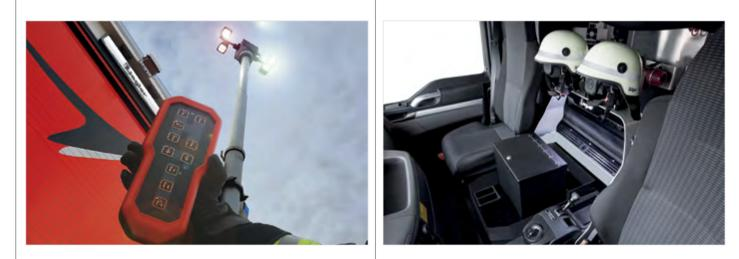
Light mast/Z-Control-Light mast control Designed for the use with gloves – safe in operation.
