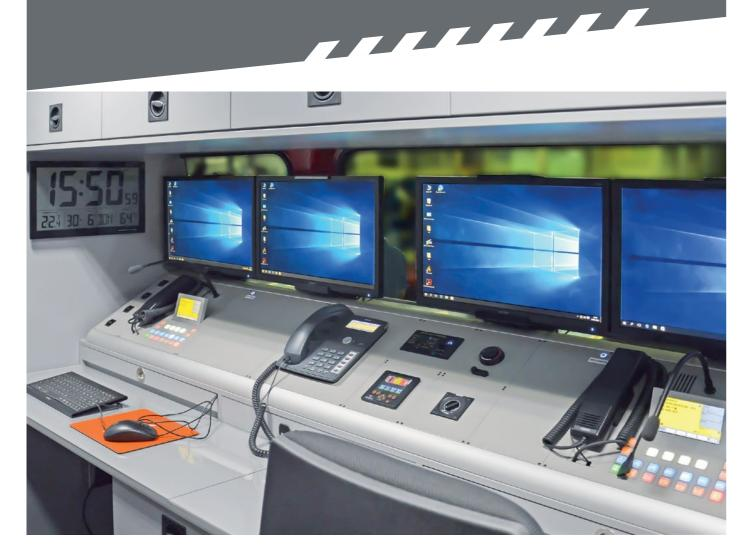
■ RADIO ROOM: Individually adapted meeting area and command center. Outfitted with the latest radio and telecommunications equipment, the ELW 1 is able to network with internal and external security organizations, thus safeguarding targeted tactical operations and communications.
