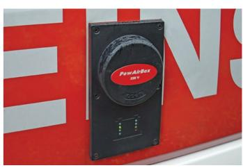
■ POWAIRBOX: The combined power and compressed air supply with automatic eject. Infeed possible with 230 V.
