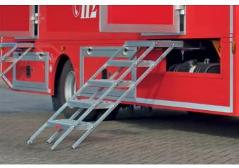
■ STOWED TO SAVE SPACE: Steps can be easily pulled out. Space-saving arrangement thanks to simple folding mechanism in the vehicle.
